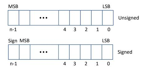
LSB = Least significant bit MSB = Most significant bit
